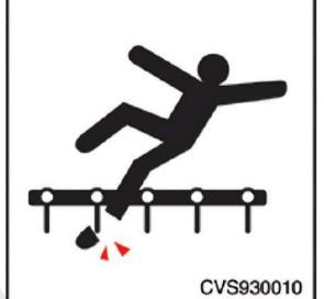
Exposed conveyors and moving parts can cause severe injury
