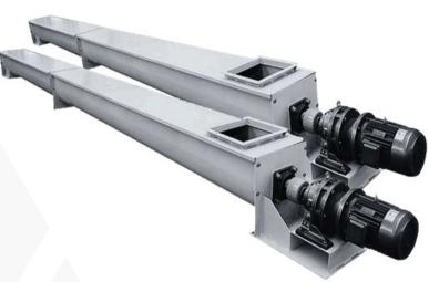
**Inclined Screw Conveyors** Used to move materials at angles up to 45 degrees. Efficiency decreases and horsepower requirements increase with steeper inclines. Suitable for conveying materials with varying degrees of incline.
